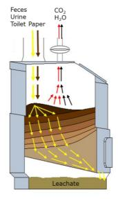
containing the kind of minerals you find in ordinary soil. If the usage compared to the size of the tank is adequate, the compost can remain in the container for several decades.
